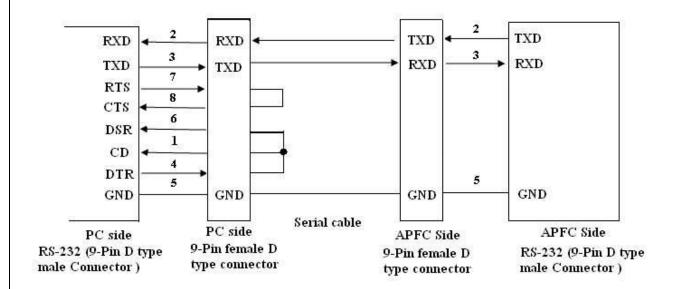
The above wiring diagram of the RS-232 Serial Communication Cable which is meant for communication between:
